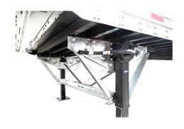
Fully galvanized, bolt-together landing leg bracing spanning seven cross members
